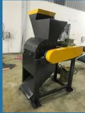
Crusher With Damaged Fly Ash Brick, Solid Block, Pavor Block And Hollow Block
