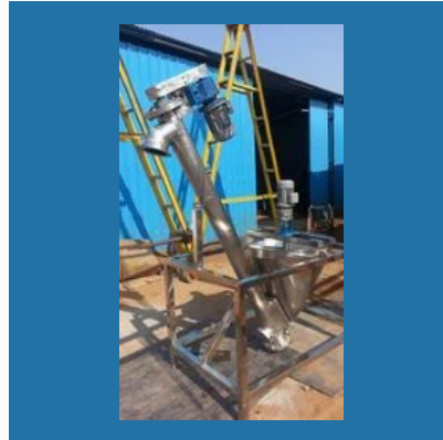
SS, MS Inclined Conveyor
